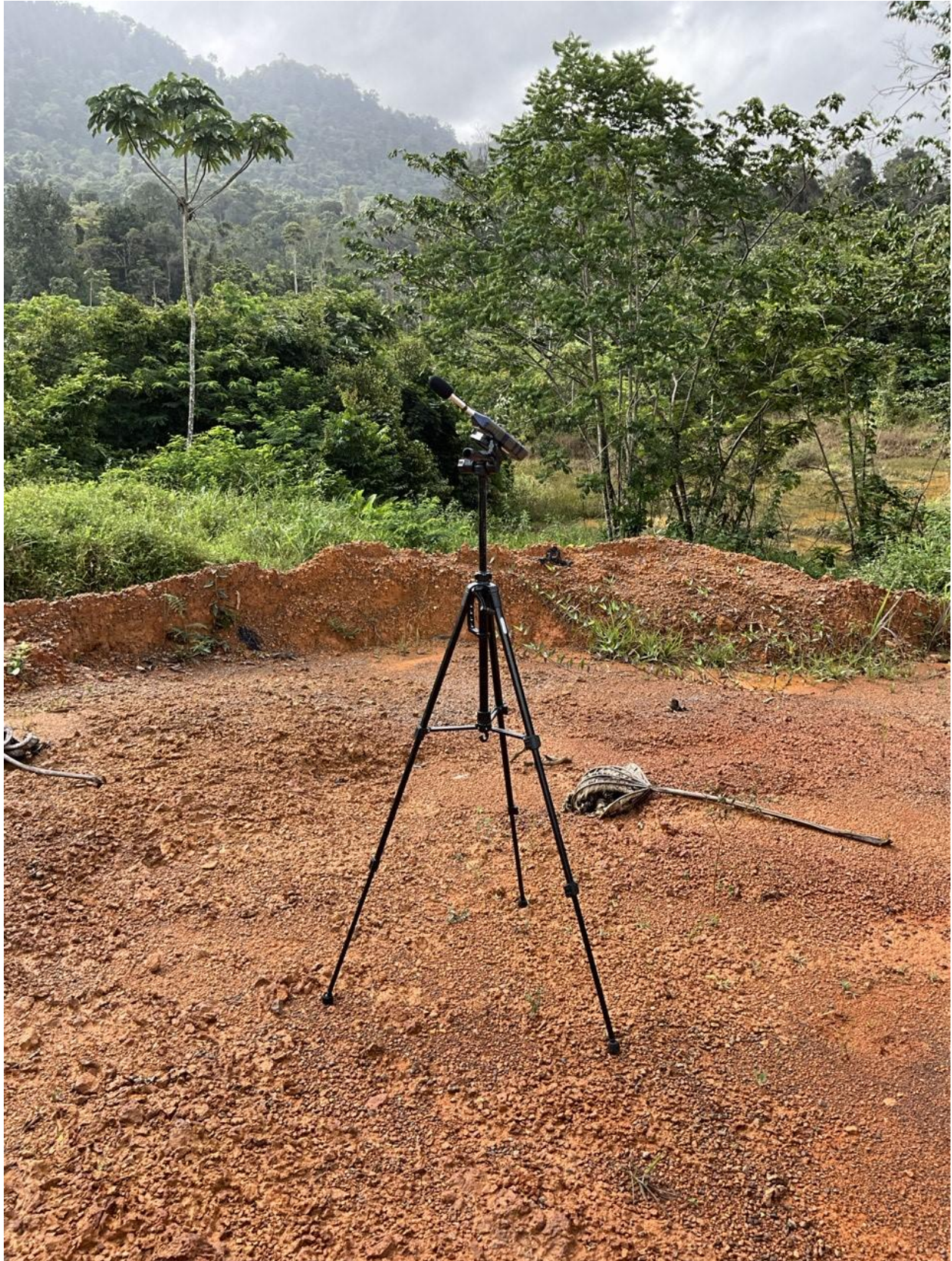
FIGURE 3.1 NOISE MONITORING SETUP
